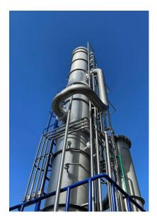
ClearAlc uses a patented highly energy-efficient, single pass vacuum distillation process capable of separating different volatile aromatic compounds (heads, hearts, and tails). ClearAlc is capable of dealcoholizing as desired down to 0.05% abv, and rectification of the alcohol fraction (up to 92% abv). ClearAlc's design uses advanced technologies to ensure sustainability with very high energy efficiency, lower maximum temperature, and minimal water use.
