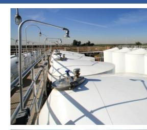
"The insulation on the tanks allows us to quickly chill and easily maintain the optimum wine temperature in any weather. Due to the fact that we insulated approximately 20% of our outside tanks each year, over the last five years, we have experienced a noticeable reduction in our PG&E bill for the same time period."
